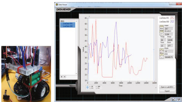
Fig. 9 Line graph of motor encoder as a function of time
